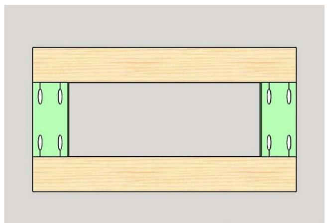
Cut 4 pieces of 1×2. Drill several countersink holes on the edge of each piece. Also, drill 3 holes in the side of each piece. Apply glue to the edge, position on the inside of the wing frame and clamp. Attach using wood screws. Repeat for the other pieces.
