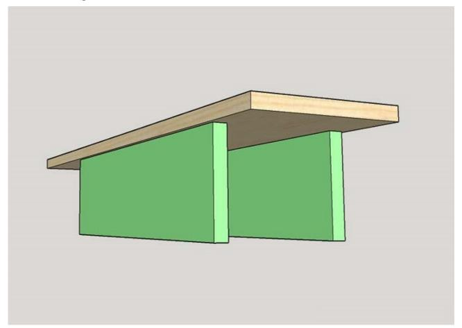
The wing table supports are based on the length of the wing table. Measure from the side of the wing table that will extend over the base of the stand to the outside edge of the  $1 \times 6$ . Then, subtract a  $\frac{1}{4}$ " from this measurement.
