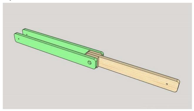
Attach 2 anchors to the upper arm. Insert a bolt with a washer into the upper arm hole and attach using another washer and a lock nut. Vighten the nut but leave it loose enough so the arms can move freely. Repeat for the other set of arms.
