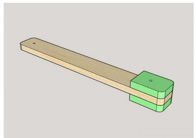
Next, I marked the location for the arm locks on the top and bottom side of the arm. I'll use these marks to attach the arm locks in Step 13.
