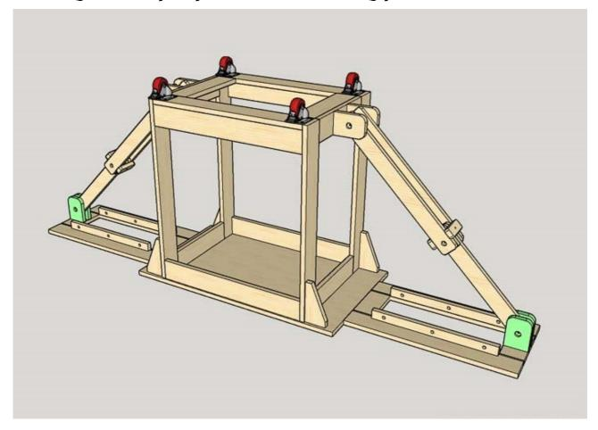
I attached 1 piece of  $1 \times 2$  to the back of the upper anchor with a wood screw. This will help push the arm in the upright position when the wing is closed.
