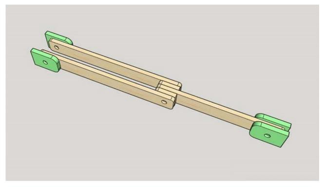
Attach the arm locks using wood screws.
