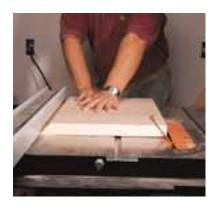
Disappearing Miter Trick • Unless your rip fence is tight to the saw table, the miter will have a tendency to slide under the fence during the second cut (on right tilt saws). Recheck your measurements to accommodate this, or add a tight-fitting auxiliary fence to the standard rip fence.
